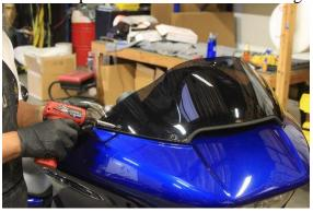
2. Remove the air duct by pulling up from the front
