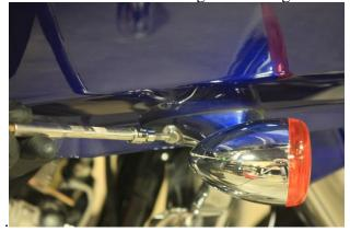
5. Remove the T-27 TORX From Under the Speaker Grill
