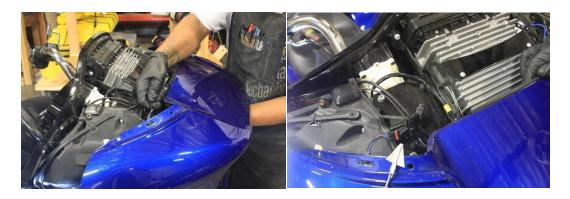
8. Remove the Radio by removing the 4 3/16 Allen head bolts at all 4 corners of the radio.
