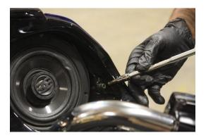
6. Remove the Lower T-20 TORX from the lower Hole on the Wind wing
