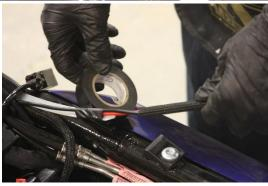
13. At the battery you will connect the power harness RED wire to the positive (+) terminal and the BLACK wire to the negative (-) terminal. The negative terminal is on the throttle side of the bike and the positive terminal is on the clutch side of the bike.
