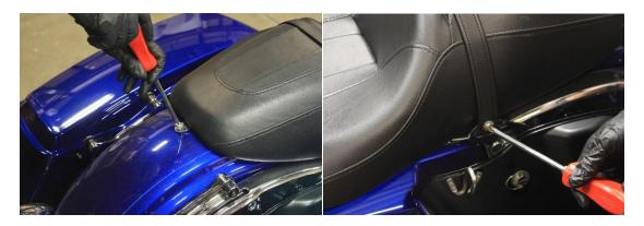
11. You will find the PCM plate under the seat. Unclip the PCM and remove the 2 T40 TORX, remove the plate.
