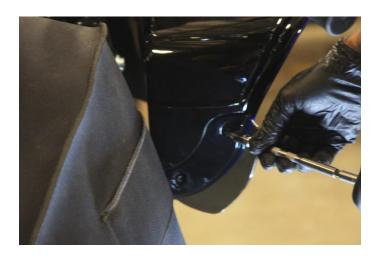
7. Disconnect turn signal plugs and Slide Outer Fairing away from Motorcycle.
