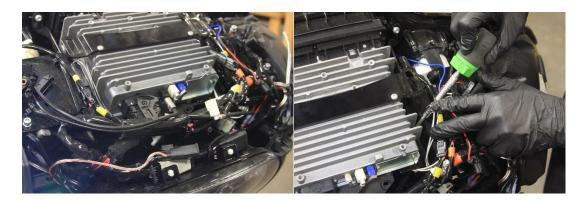
9. Remove the Headlight by Removing the 4 3/16 Allen Head Bolts Remove the 2 plugs attached to the top of headlight.
