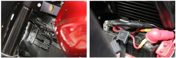
Feed end of Amp harness into fairing alongside existing wiring loom to battery.
