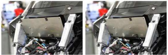
Set speed clips in position for 2 or 4 channel Amp.
