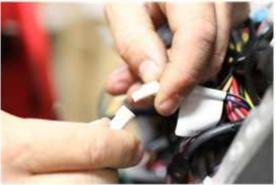
Disconnect headlamp and set aside.Unplug turn signal wires.
