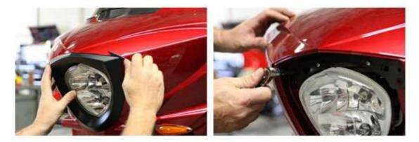
Using pocket nice knife, separate trim bezel.Remove headlight with 5mm allen wrench.
