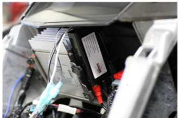
Attach new connectors to speaker wire and attach Line level converter. Left front (+) Dark Grey w/ Red tracer to White Left front (-) Brown w/ Black tracer to White / Black Right front (+) Light Grey w/ Red tracer to Grey Right front (-) Light Grey w/ White tracer to Grey / Black
