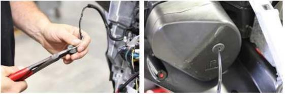
Pull existing speaker wire and cut rubber speaker grommet.
