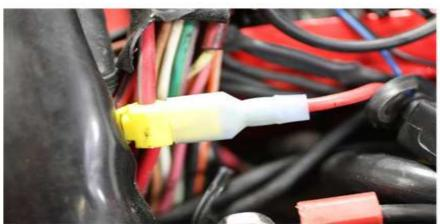
Standard radio: Yellow - positive battery terminal through fuse holder.
