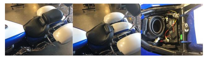
2) Remove rear tank bolt and place roll of electrical tape under tab to lift
