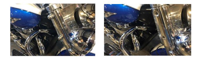
2) Slide fairing onto OEM Windshield Inner grommets. Plug in all connections at this point.
