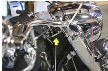
7. Connect wires as follows: Red - Crimp provided in line fuse to wire and attach to positive side of battery \*\*do **not install fuse at this time**\*\*. Black – Crimp provided ring terminal to line and attach to negative side of battery. Blue – locate wire that is powered only with the ignition on and attach the provided t-tap to the wire. Crimp male spade to blue wire and connect to the t-tap.
