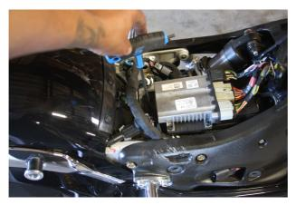
6. Run a fishing tape or line to allow the provided harness to be pulled through. Start in front of bars on throttle side and route down the side of the neck, under the tank coming out near battery.
