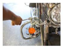
3. Install relocation brackets with the provided 3/8 X 1" bolt and Nylok® nut as shown. Reattach spotlight.
