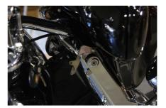
9. Lower locking tabs into place and install 8/32 X <sup>1</sup>/<sub>2</sub>" screws and Nylok(s)® to secure fairing.
