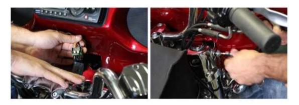
Align bottom slots on bracket with bottom windshield bolts.
