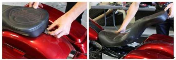
cover fuel tank and front fender to prevent scratches during install - remove seat and set aside
