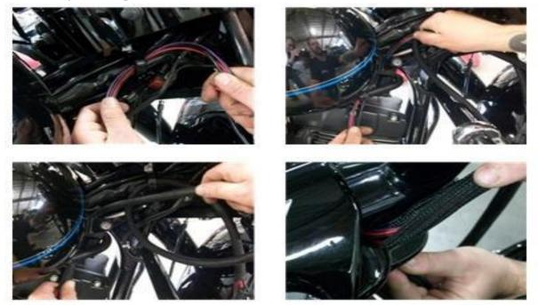
4) Harness(s) should <u>exit</u> near battery. Attach wires per guide.
