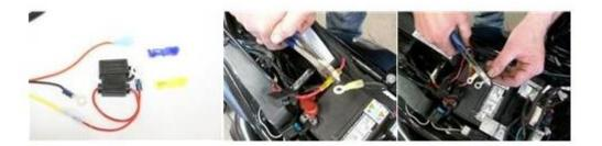
Standard radio: Yellow 16ga- Attach fuse holder and connect to Positive battery terminal Black 16ga- Negative battery terminal
