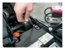
2) Remove rear tank bolt and place roll of electrical tape under tab to lift
