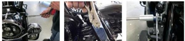
2) Using 5/32 ball socket allen wrench, remove turn signal.
