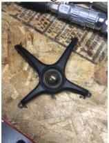
3. Once you have done that flip it upside down and remove the screws from the existing tweeter and pop it out the bottom.
