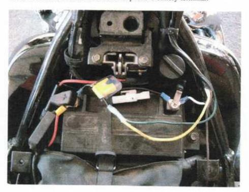
15.) Locate the blue wire running along the left side of the frame behind the battery. Connect the brown wire from the quick disconnect harness to the blue wire.
