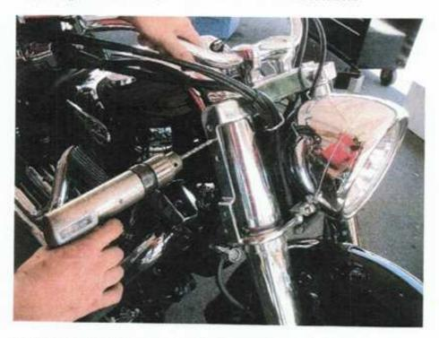
13.) Run the quick disconnect wiring harness down the right side of the frame starting at the steering head and working back under your fuel tank to the battery. You may find it helpful to loosen the rear fuel tank mount and lift the rear of the fuel tank slightly.
