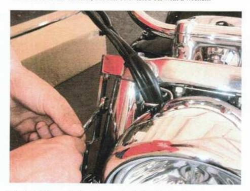
11.) Using the supplied template, mark the location for the fairing bracket bolt holes with a center punch.
