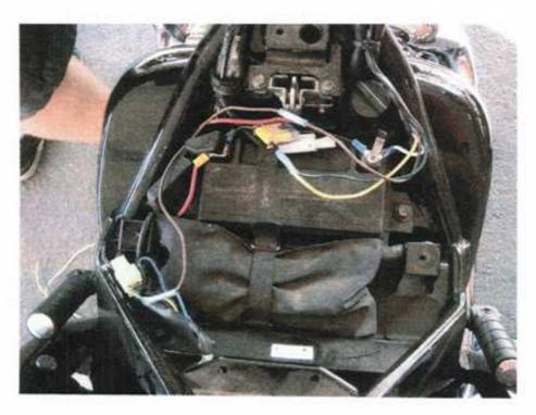
16.) As you bring the fairing to the motorcycle, attach the four prong connector from the quick disconnect harness to the four prong connector from the radio. Attach the fairing to the motorcycle with the supplied bolts and nylok nuts. The fairing brackets should be positioned to the inside edge of the factory windshield brackets.
