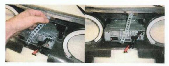
5.) Plug in the antenna wire and the radio wiring harness, which supplies power and connects both speakers. Zip tie the antenna to the backstrap on the top side of the stereo.
