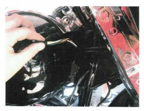
14.) At the battery, connect the white wire to the negative battery terminal. Connect the yellow and green wires together with the butt connector attached to the supplied fuse. Attach the other end of the fuse to the positive battery terminal.
