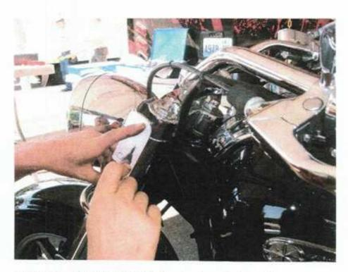
12.) Using a 3/8" drill bit, drill holes at each marked location.
