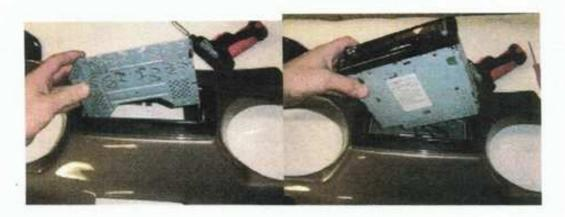
4.) Use the supplied stereo back strap to hold stereo in place. Attach one end to the 3/16" hole on the inner fairing center windshield bolt support, and the other to supplied bolt on the back of the stereo.
