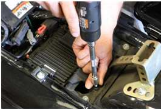
-Remove access cover to battery
