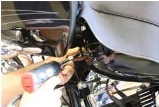
-Remove tank bolts and disconnect fuel lines - Cover tank and set aside
